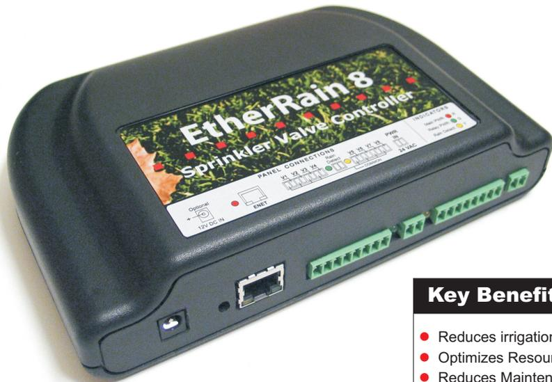
EtherRain 8 - Controls up to 8 Valves
